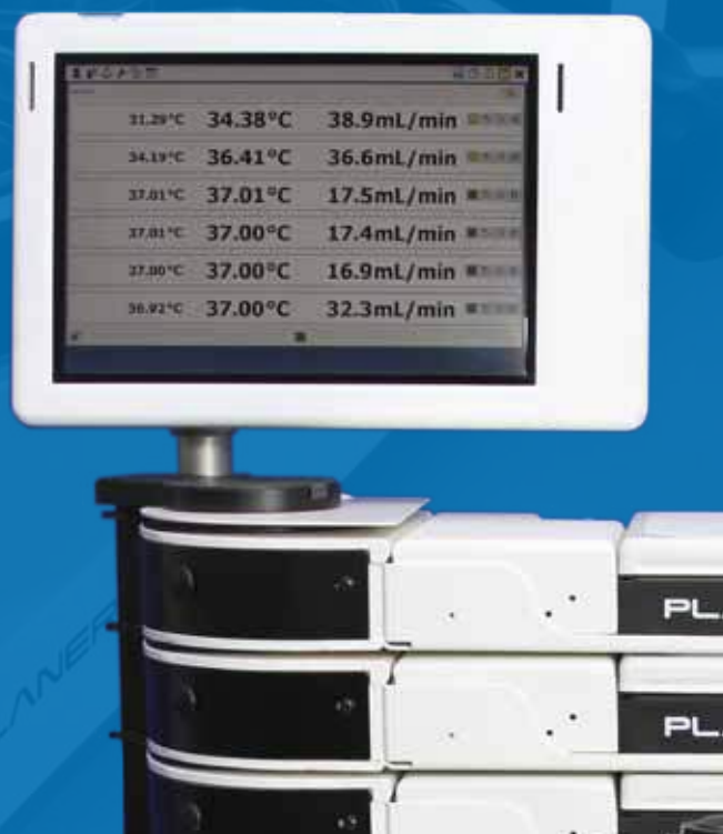
PIMSsolo unit mounted on a CT37stax™ system
